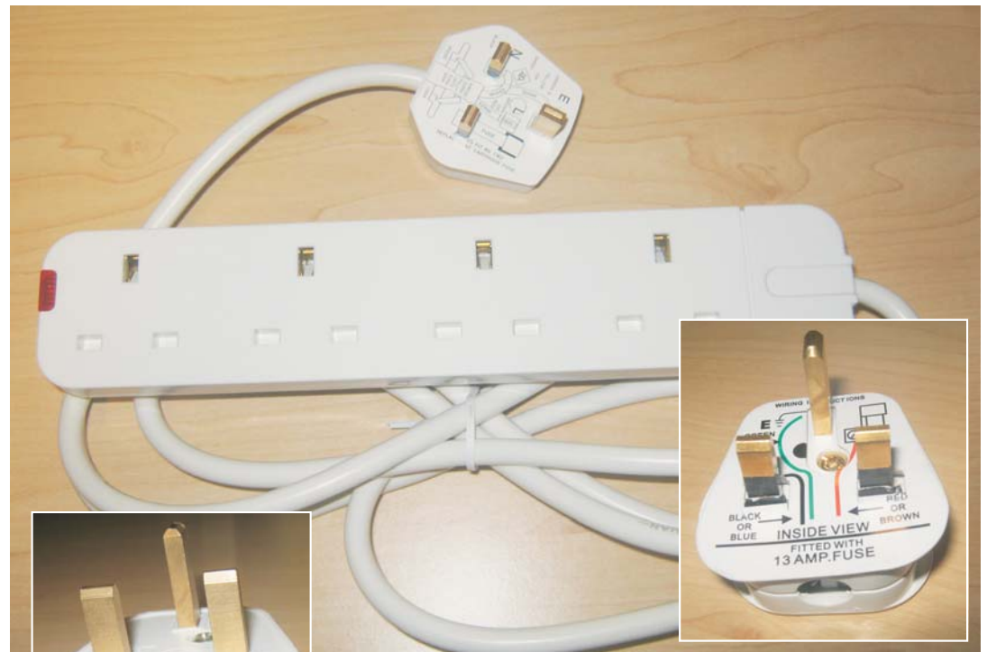
Non-compliant and compliant plugs (visual inspection). The plug on the left has no wiring instructions and no insulation sleeves on the live and neutral pins. Above: Compliant portable socket outlets with shutters where the plug is inserted.
