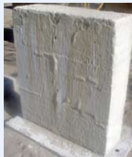
Figure 3 - Test wall 3 (95% gravel + 5% cement stabilizer).
