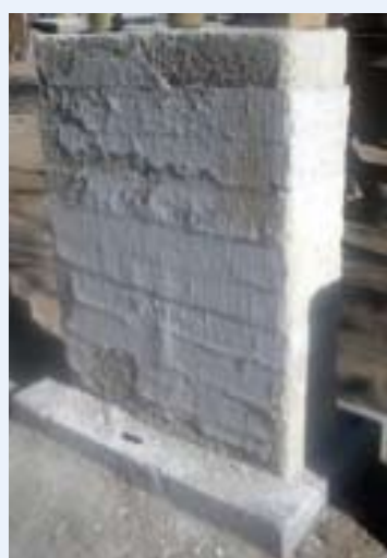
Figure 2 - Test wall 2 (90% gravel + 10% cement stabilizer).
